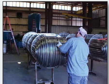
Assembling removable 'U' tube bundles for 'BJU' Type Shell & Tube Heat Exchangers.
