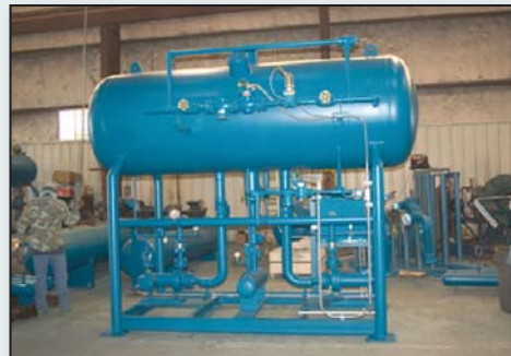
Separator vessel with pumps and controls.
