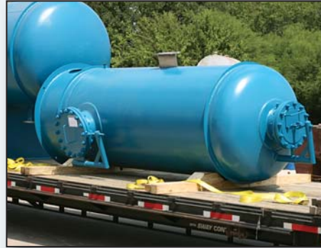
48" Dia. x 8' 0" Vertical Reflux Accumulator
