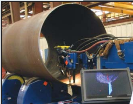
Submerged Arc Welder
