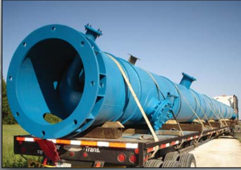
60" Dia. x 60' 0" Vertical Still Vessel
