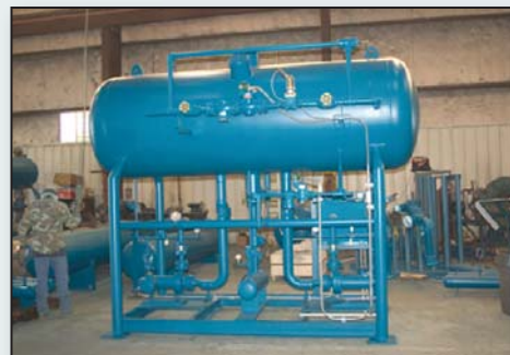
Separator vessel with pumps and controls.
