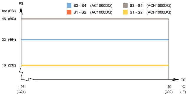
**AC1000DQ / ACH1000DQ - UL approval pressure/temperature graph**
