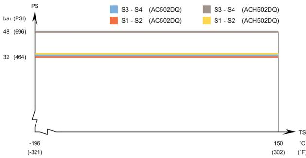
AC502DQ / ACH502DQ - UL approval pressure/temperature graph
